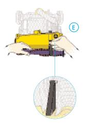
**E** Use back of cleaner as lever, loop belt around thumb. Turn the belt 90 degrees, stretch and release over spindle.
